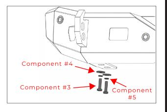
5. Position stud plate inside the frame rail and loosely attach M12 nut from the side.
