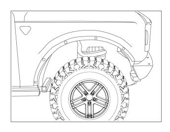
6. Replace fasteners and screws removed in Step 2 to reattach fender liner.
