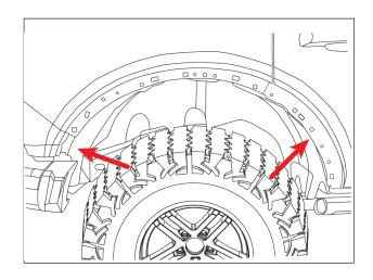
9. Install fender delete using (5) 133606M bolts, (10) WA1-0029 washers, and (5) NU1-0015 nuts. (See diagram below)
