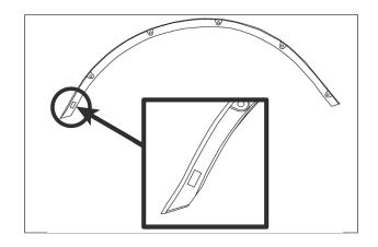
5. Install fender delete using (5) 133606M bolts, (10) WA1-0029 washers, and (5) NU1-0015 nuts. (See diagram below)
