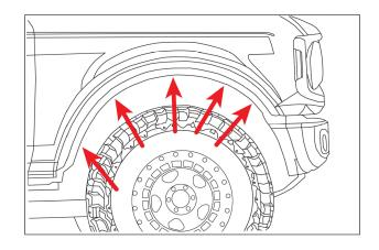
2. Remove and retain (4) factory plastic fasteners and (3) factory screws to access backside of fender.
