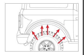
8. Remove (2) fender liner fasteners and retain.
