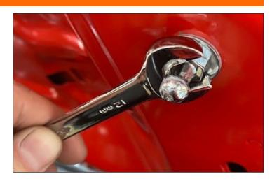
7. Install strut with piston rod pointed down. Install on hood ball socket, then on fender. Repeat steps on passenger side.
